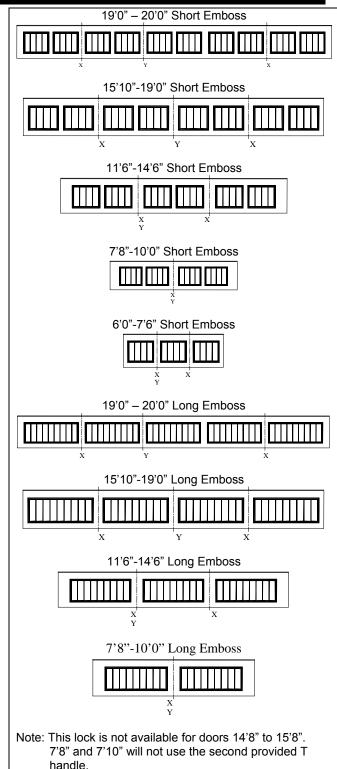
FIG. B – Configuration of Handles for Hole Drilling Placement
