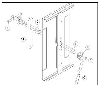
FIG. C – Assembly of Keyed Twisted "T" Handle (Uninsulated Door Shown)
