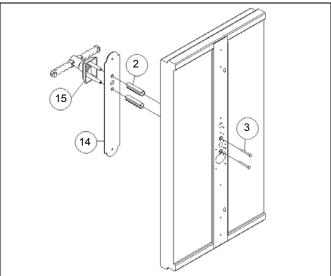
FIG. D – Assembly of Nonworking Twisted "T" Handle (Insulated Door Shown)
