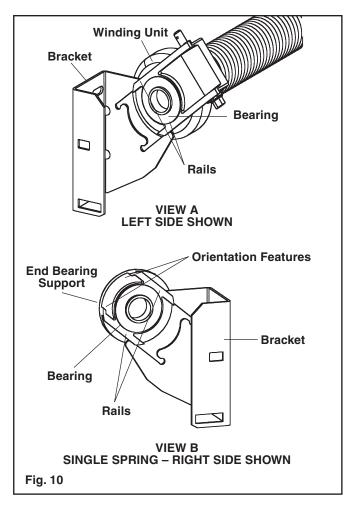
NOTE: The drums and torsion tube are removed from Figure 10, View A and Figure 10, View B for clarity.
