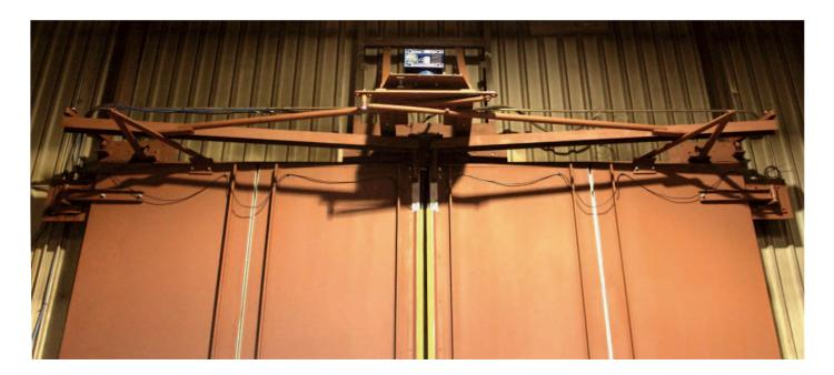
**Door Construction** - Doors are constructed of an 11 gauge structural steel tube frame and 18 gauge steel sheeting formed around vertical edges to provide smooth aesthetic finish. Sheeting is bonded to a 1-1/2" extruded polystyrene core.
