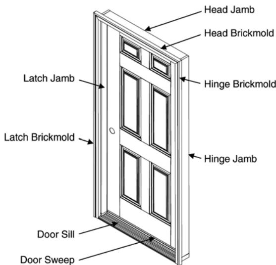
**IMPORTANT: Before setting the door unit into the rough opening, apply generous beads of caulk to the underside of the door sill at locations shown in figures 1a or 1b and include the plastic sill key and brickmould. Apply at least 4 lines of bead caulk over the full width of the subfloor sill area. Also apply a continuous and generous bead of caulk to the back side of each brickmould as shown in figure 1c.**
