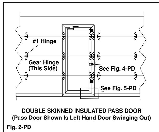
NOTE: Swinging portion of Pass Door on bottom section may need to be shimmed up during installation of upper sections to prevent gapping. (FIG. 5-PD)
